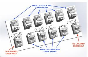
Insert check rails into shared sockets to complete both stock rail assemblies.
