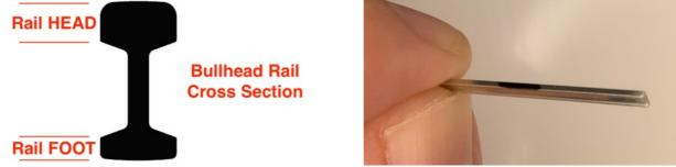
• Ensure all rail ends are deburred. It's a good idea to file a tiny lead in chamfer to both ends of rail to enable chairs to be easily threaded onto rail.
