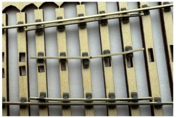
• Thread 2<sup>nd</sup> Wing Rail through datum knuckle chair. Thread remaining split wing chairs onto 2<sup>nd</sup> wing rail. Test fit pair of Wing Rails into ply timbers.
