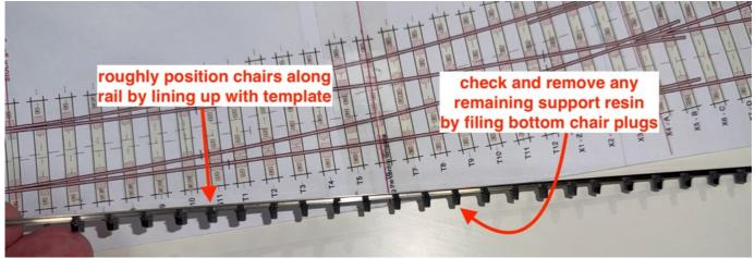
Starting at one end, align and partially insert first chair into respective timber socket. Hold rail in place at
