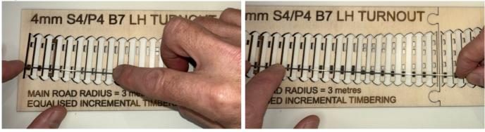
• Whilst holding down rail and first inserted chair repeat the slide/wiggle/twist routine to partially insert remaining chairs. The fit of the chairs is almost size for size so minimal force is required. As more chairs begin to be inserted the first chairs can gradually be pressed home.
