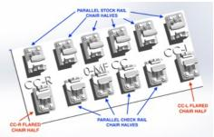
• As chairs are threaded onto rail ensure all keys are fitted on the outside of the rail. Key direction along the rail should be random apart from chairs adjacent to a gap/fishplate/joint where keys would prototypically be fitted facing away from rail joint. (I need to check / confirm this?)
